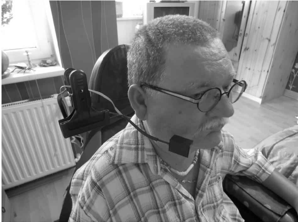
Fig. 1. An example of installing sensor type “A” at a distance of 7 cm from the operating person’s face
