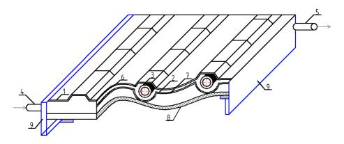
Fig. 1. Scheme of solar roof: 1 - top hose cover, 2 - bottom hose cover, 3 - tube circuits,
