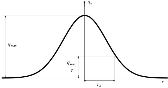
Fig. 1. Gaussian distribution of volumetric heat source
