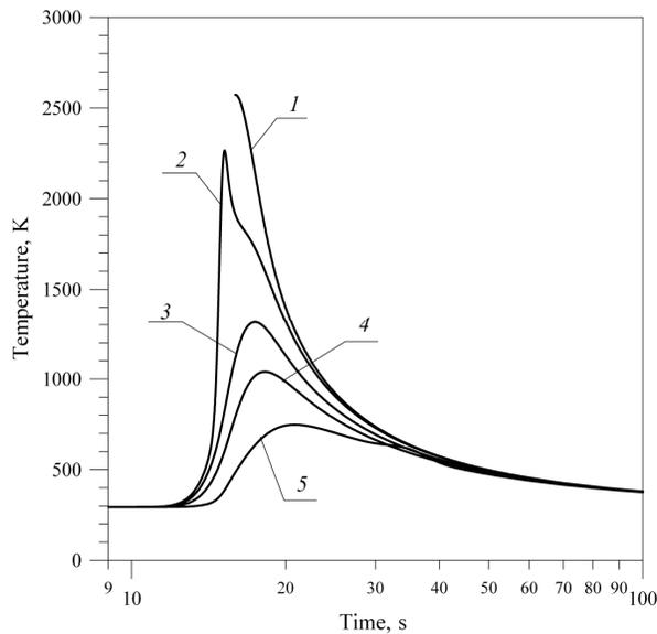
Fig. 9. Thermal cycles at selected points of cross-section
