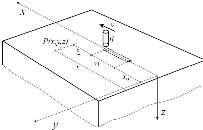
Fig. 2. The scheme of single-pass surfacing
