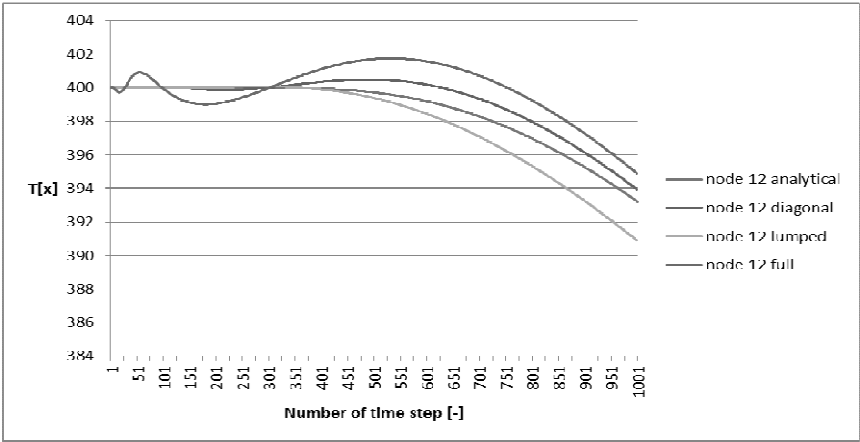
Fig. 5. Temperature dependency on the time for node 12
