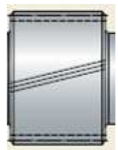
Fig. 9. Representation of gear with simplification
