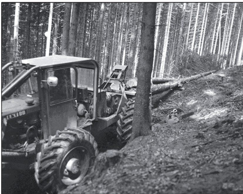
Phot. 3. The wheels of forest tractors damage the roads and slopes around (phot. by L. Buzek)
