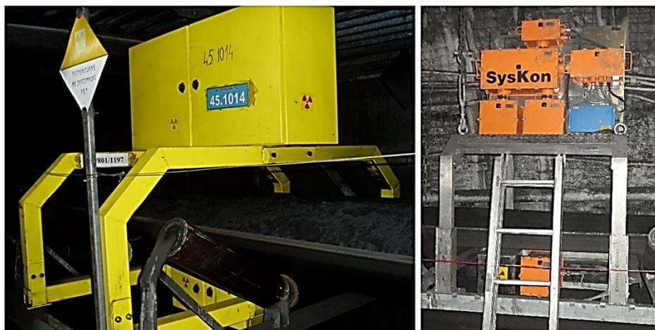
Fig. 4.8. SysKon400, the system for a continuous control of coal qualitative parameters in the LW Bogdanka SA (Dyczko *et al* 2015)
