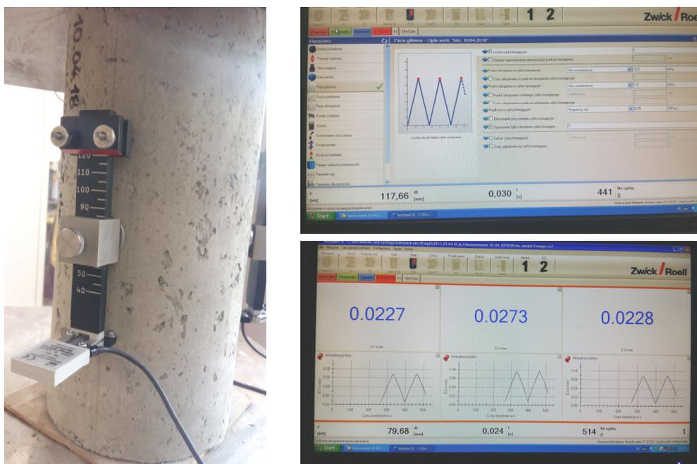
Fig. 2. Sample (150x300 mm) during the test and the screenshots (from testXpert program) of the results from the Young's module measurement (*own study*)
