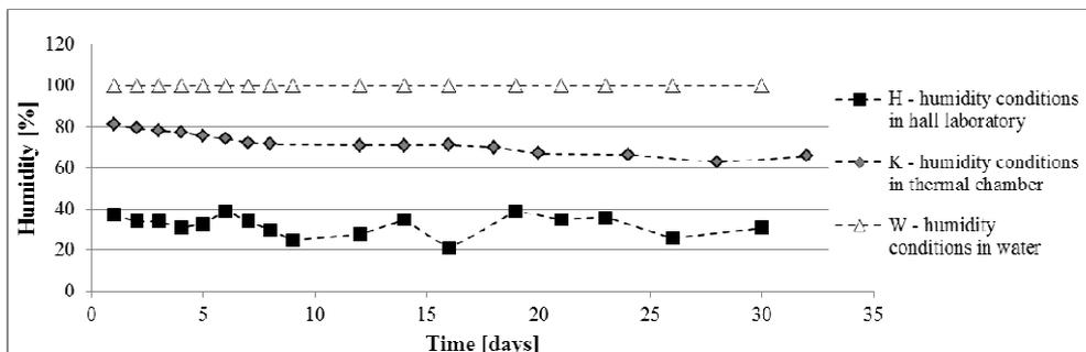
Fig. 1. Graph of relative humidity measured during the tests (*own study*)
