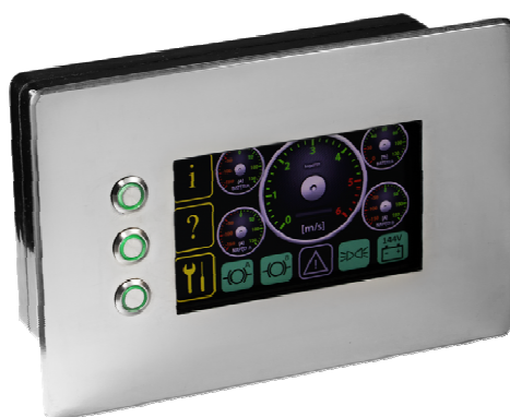
Rys. 1. Panel operatorski PO-1 [29]
