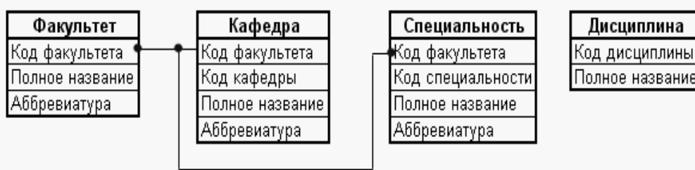
Figure 1 – The IRS core structural scheme
