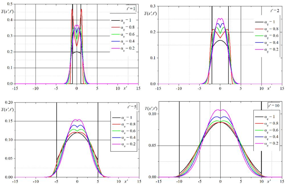
Fig. 2. Effect of fractional order  $\alpha_q$  on temperature distribution  $T(x', t')$  over space at the selected moments of time  $t' \in \{1, 2, 5, 10\}$
