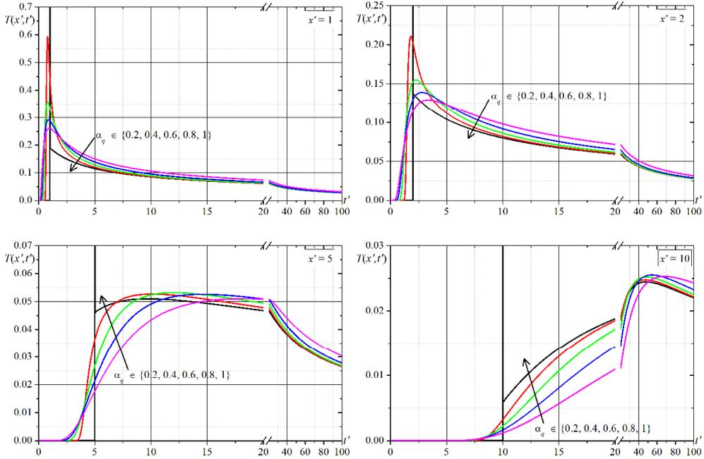
Fig. 3. Effect of fractional order  $\alpha_q$  on temperature distribution  $T(x', t')$  over time at the selected points  $x' \in \{1, 2, 5, 10\}$
