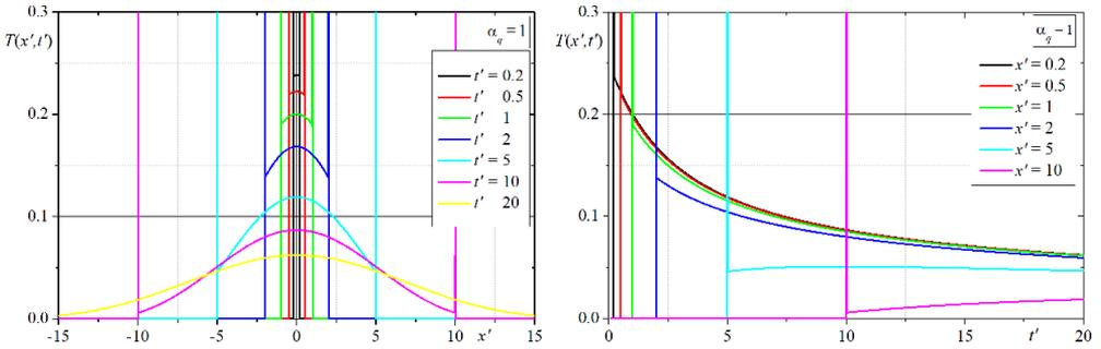
Fig. 1. Temperature distribution  $T(x', t')$  over space and over time for  $\alpha_q = 1$  (classical Cattaneo equation)
