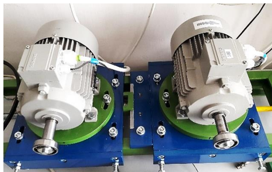
Fig. 2. Test bearings mounted on the experimental stand
