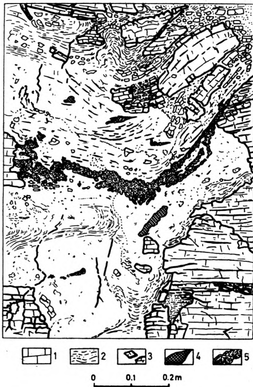
Fig. 6. Example of a filled karst channel (Olkusz ore-mine):
