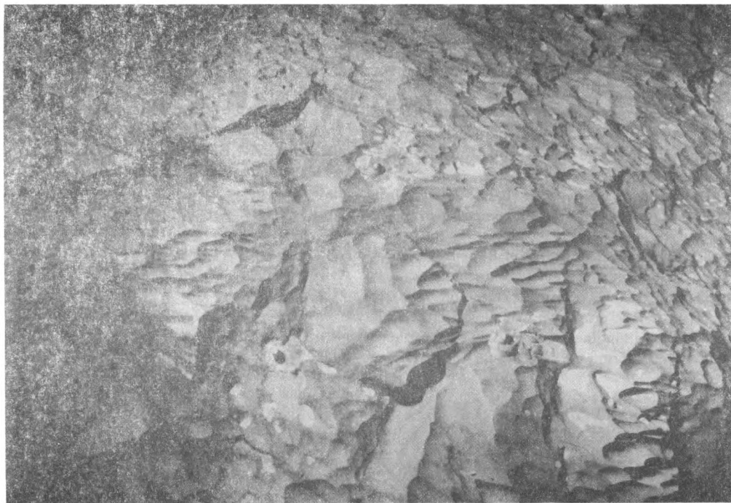
Photo 2. The surface of the current markings net. They are long and narrow showing extreme flow velocity. In the middle of the picture there are three studs on which the micrometer is placed, the distance among them is 15 cm
