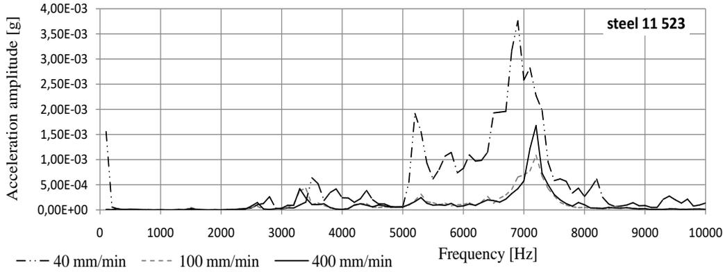
**Fig. 6.** The technological head vibration frequency spectrum envelopes when cutting the 11 523 steel
