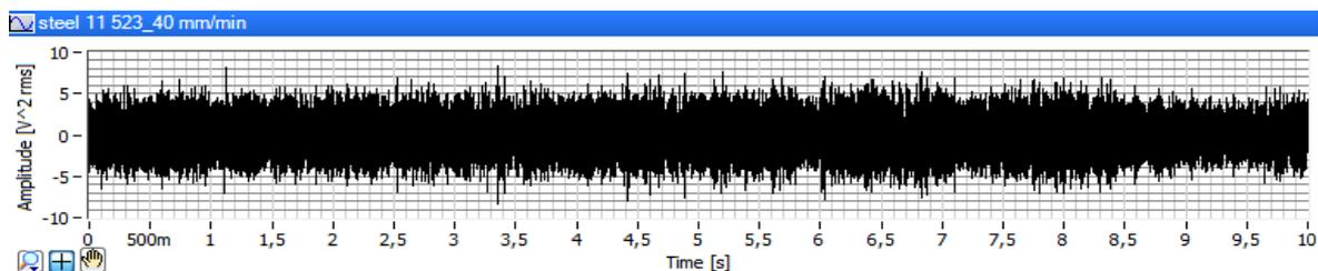
**Fig. 3.** A time record of the vibration acceleration amplitude of 11 523 steel cutting at a feed rate of 40 mm/min
