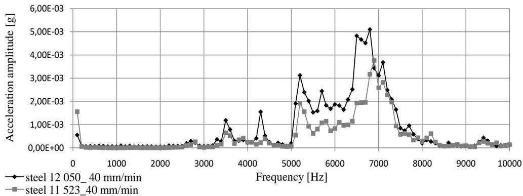
**Fig. 7.** The technological head vibration frequency spectrum envelopes comparison at the cutting feed rate of 40 mm/min
