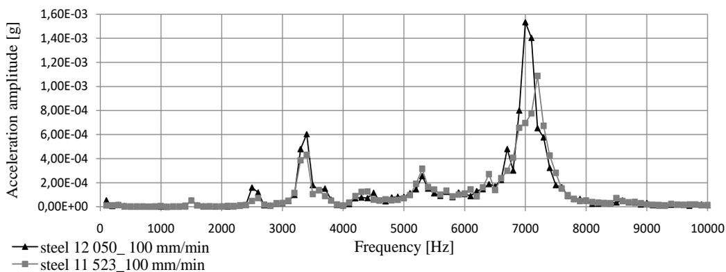
**Fig. 8.** The technological head vibration frequency spectrum envelopes comparison at the cutting feed rate of 100 mm/min
