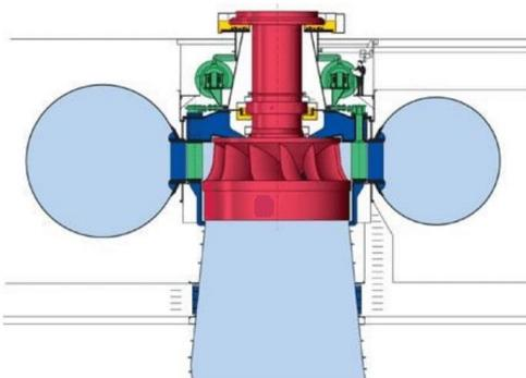
**Fig. 4.** Schematic diagram of Francis turbine [29]
