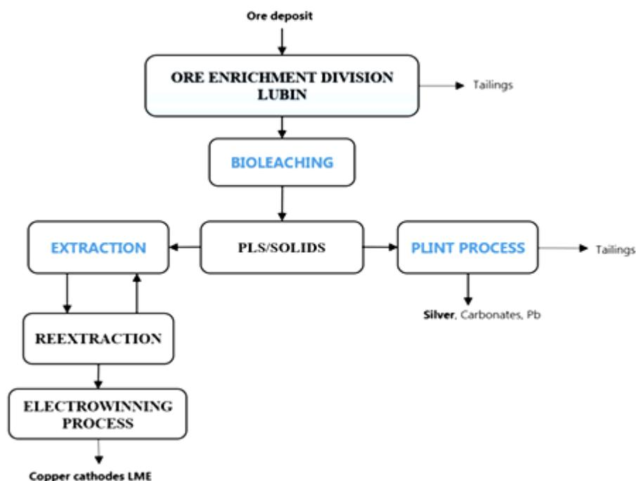
Fig. 2. Simplified diagram of Bioshale technology [25]
