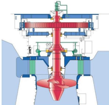
**Fig. 2.** Schematic diagram of Kaplan turbine [27]
