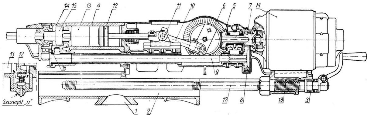
Fig. 1. Mine electric rotary - percussion drilling machine Pneumelectric [2]
