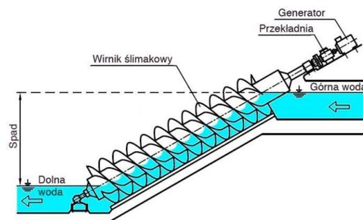
**Fig. 5.** Schematic diagram of Archimedes turbine [30]
