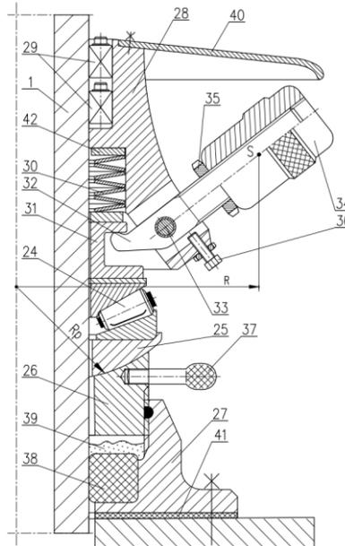
Fig. 8. System that relieves the plain bearing [38]
