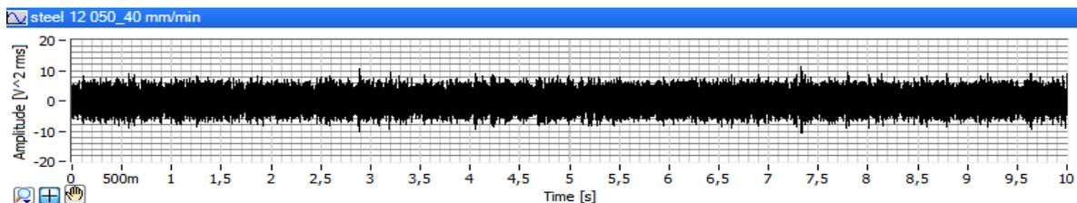
**Fig. 2.** A time record of the vibration acceleration amplitude of 12 050 steel cutting at a feed rate of 40 mm/min
