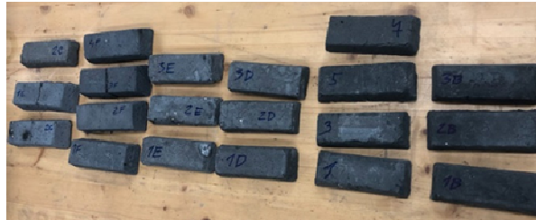
Fig. 2. Part of the manufactured experimental geopolymer samples ( own research )
