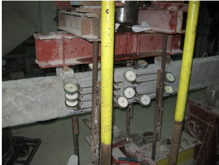
Fig. 3. General view of test samples installed on the test stand for short-term bending load ( own research )
